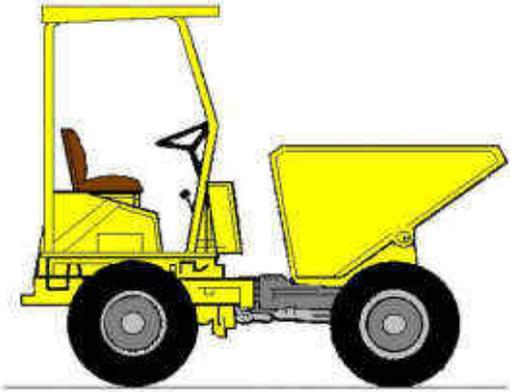
A side-view illustration of a yellow motorized dumper truck. The truck has a large, yellow, conical hopper at the rear for dumping material. The operator's seat is on the left side, with a steering wheel and a protective roll-over structure. The truck is shown on a simple grey ground line.                                                                                                                                    |                  |
